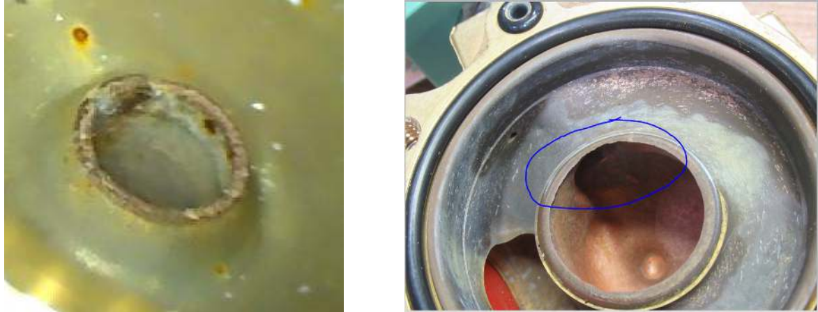
Examples of eroded valve seats exhibiting wire draw (left) and as result of dezincification (right)
