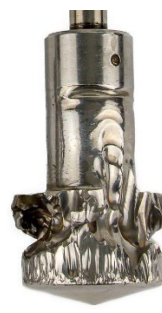
Control Valve Plug with Flashing Damage
